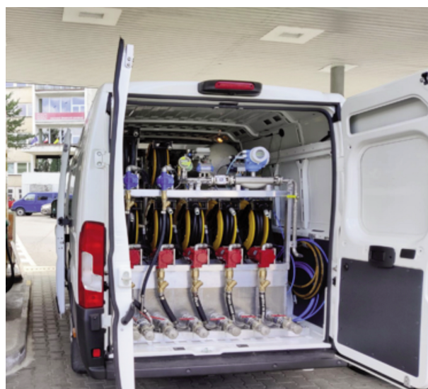
Fig. 15 Ways of emptying the measured liquids (by gravity or pump)
