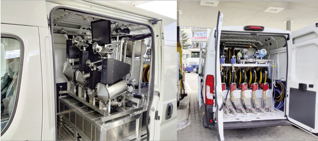
Fig. 1 MCoFD system as a part of the vehicle for verification
